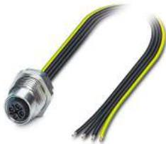
Device connector, rear mounting, Power, 4-position, Socket, straight, M12, coding: S power , on free cable end, Rear mounting, M16 x 1.5, Individual wires, cable length: 4.5 m, 1.31 mm<sup>2</sup>, UL/cUL stranded hook-up wire, Alternative product in accordance with RoHS II without Exemption 6c (Pb <0.1%) item no.: 1239295
