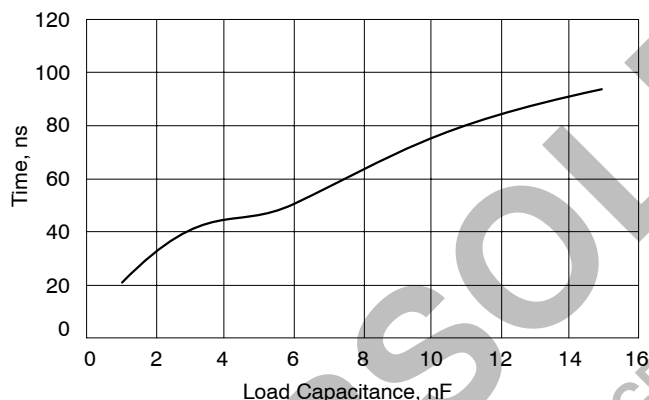
Figure 5. GATE(H) Rise-time vs. Load Capacitance measured from 1.0 V to 4.0 V with V CC at 5.0 V.
