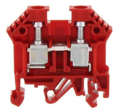
Feed-through terminal, Screw connection, Mounting type:Mounting rail TS 35/7.5 and TS 32, Rated cross-section: 10 mm<sup>2</sup>, Width: 8 mm, Colour: Red
