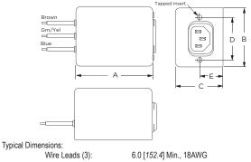
Wire Leads (3): Line Inlet (1): Q8 Tapped Inserts (2): Q8M Tapped Inserts (2): 6.0 [152.4] Min., 18AWG IEC 60320-1 C14 6-32 x 1/4 M3 x .5
