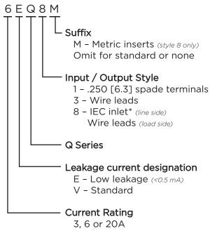
\*IEC 60320-1 C14 inlet mates with C13 connector
