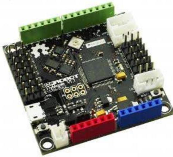
Flymaple is a Quadcopter controller board, based on the Maple Project. The FlyMaple embeds a STM32F103RET6 (ARM Cortex-M3) as it's main MCU. It integrates a 3-Axis accelerometer,a 3-Axis gyroscope,a 3-Axis compass and a barometric pressure sensor. By using the 10 degrees of freedom IMUs and powerful 72MHz high-performance microcontroller, flymaple is powerful enough to handle a complex algorithm and manage a robot motion system at the same time.
