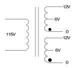
\* Secondary windings are designed to be connected in series or parallel. Windings are not intended to be used independently.
