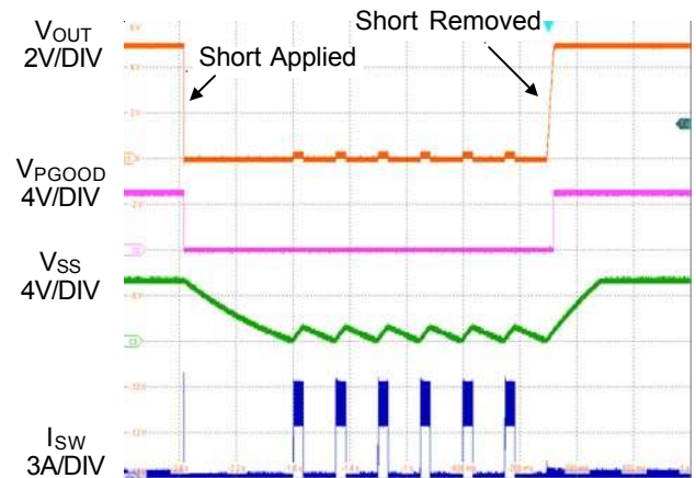
Figure 3. Short-Circuit Protection and Recovery
