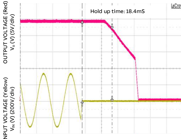
Figure 7. Typical Hold-up Waveforms ( V_{IN} = 230\text{V} , 100% Load)
