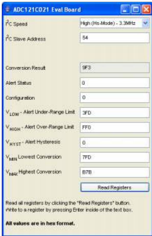
Figure 10: ADC121C021 Control Panel
