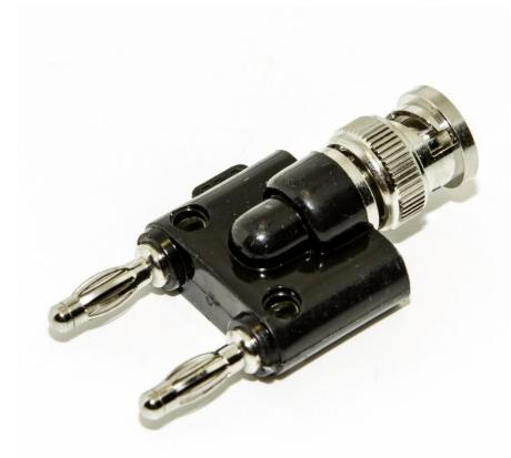
• The BU-P1270 is a dual stacking 4mm banana plug to male BNC. Allows a BNC female connector to be converted for use with standard 4mm banana jacks spaced 0.75" center-to-center.
