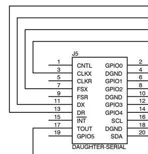
J5A (TOP) = SAM_TSM-110-01-L-DV-P J5B (BOTTOM) = SAM_SSW-110-22-F-D-VS-K
