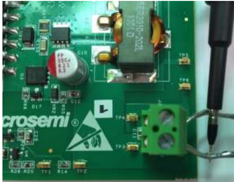
Figure 11. Proper ripple measurement
