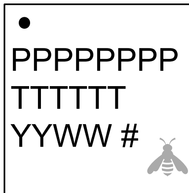
Figure 10.3. QFN24 Package Marking
