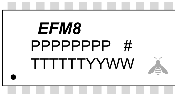
Figure 11.3. QSOP24 Package Marking
