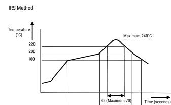
Note: Temperature profile shows printed circuit board surface temperature on the relay terminal portion. Please consult KEMET if you wish to use a temperature profile other than above.
