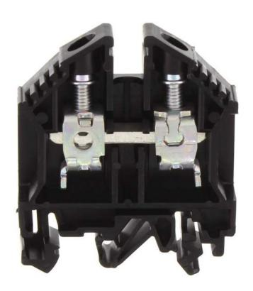
Feed-through terminal, Screw connection, Mounting type:Mounting rail TS 35/7.5 and TS 32, Rated cross-section: 16 mm², Width: 12 mm, Colour: Black
