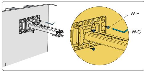
Using 5mm allen key (W-C), attach the mounting bracket to the wall plate with screws (W-E).
