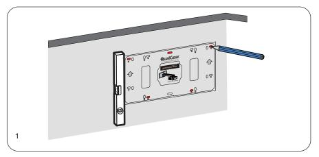
Hold the marking template against the wall where you want to install the projector, mark five holes for drilling.
