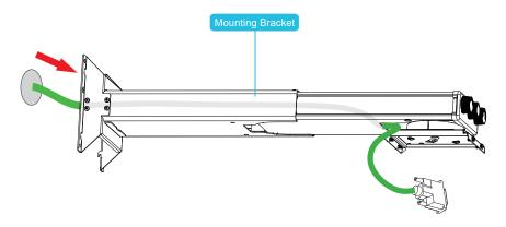
Feed the projector cable(s) through the mounting bracket.
