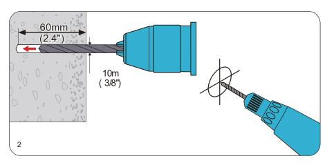
Using a power drill and a 3/8" masonry drill bit, drill mounting holes of 3/8" (10 mm) diameter and 2.4" (60 mm) depth at the marked locations in the previous step.
