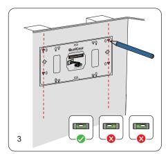
Using the marking template provided, mark four holes for drilling on the centerline of each stud.
