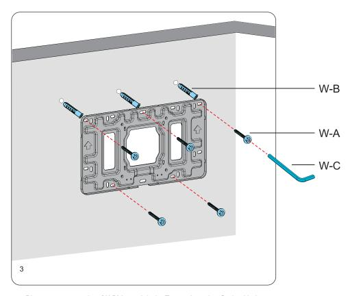
Place concrete anchor (W-B) in each hole. Tap each anchor flush with the wall using a hammer. Using a 5mm allen key (W-C), mount the wall plate and fasten with the M6x55mm screw (W-A).
