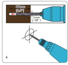
Using a power drill and 1/8" drill bit, drill pilot holes of 1/8" (3mm) diameter and at least 2.2" (55mm) depth at the marked locations in the previous step.
