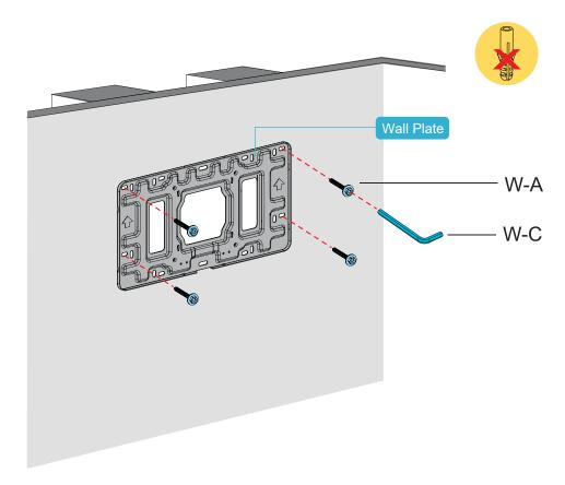
5. Using a 5mm allen key (W-C), mount the wall plate and fasten with the M6x55mm screws (W-A).
