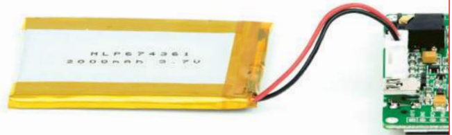
Figure 1-2: Connecting Li-Polymer battery
