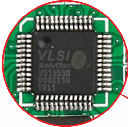
Figure 8-1: On-board VS1053 MP3 codec
