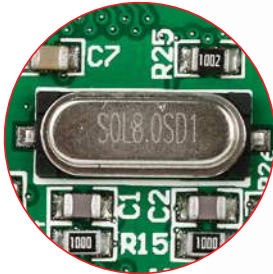
Figure 5-1: Crystal oscillator module
