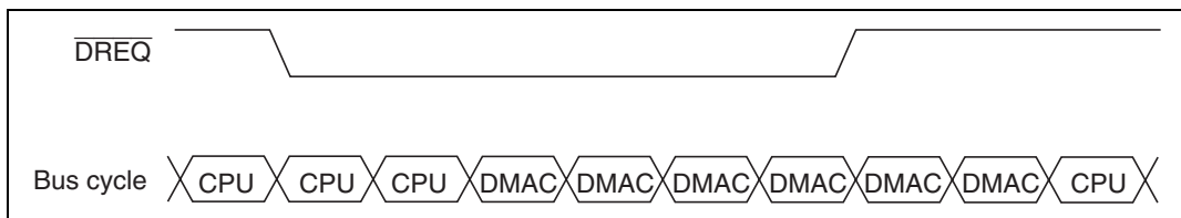
Figure 9.8 DMA Transfer Example in the Burst Mode
