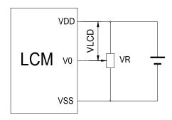
V<sub>DD~</sub>V<sub>0</sub>: LCD Driving voltage
