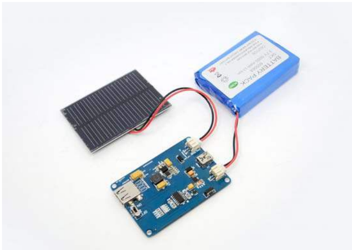
Charge Lithium Polymer Battery through solar power
