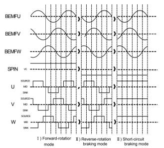
6. Motor start pattern adjustment terminal (MTR\_R)
