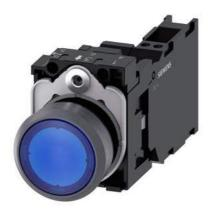
Illuminated pushbutton, 22 mm, round, plastic with metal front ring, blue, pushbutton, flat, momentary contact type, with holder, 1 NO+1 NC, LED module with integrated LED 24 V AC/DC, Spring-type terminal
