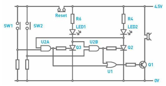
The quiz buzzer is based around two types of logic gates. There are two AND Gates and one OR Gate. Let's first examine Gate U2a. One input of the AND Gate is connected to the Push to Make Switch SW1 on the left of the circuit. These are the switches used by the quiz contestants.
