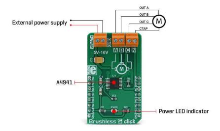
When the zero-crossing occurs, an internal signal is set to a HIGH state, while the beginning of the next phase commutation sets this signal to a LOW state. The signal is latched between the states so that commutation transients do not affect it. This provides a robust and accurate position sensing system.
