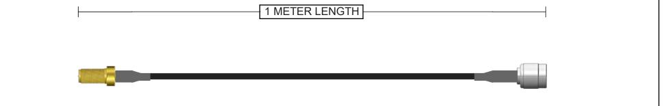
Connector A 132117RP SMA Jack Straight Brass Gold + Heatshrink 50 Ohm RG-174 Continuity/Hi-Pot Connector B 122116 TNC Plug Straight Brass Nickel IP67 + Heatshrink
