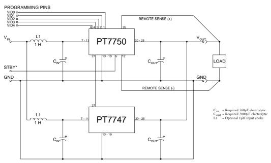
Output Capacitors: The PT7750/PT7747 series requires a minimum output capacitance of 2000µF for proper operation. Do not use Oscon type capacitors. The maximum allowable output capacitance is (42,000 + Vout)µF for the PT7751, (96,000 + Vout)µF for the PT7756, or 15,000µF, whichever is less.
