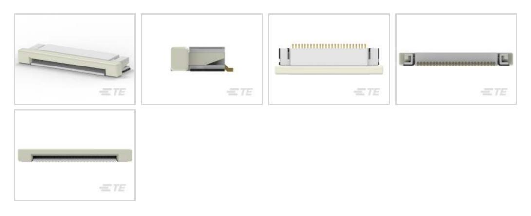
Connector System: Flex-to-Board Number of Positions: 25 Centerline (Pitch): .5 mm [ .02 in ] Insertion Force Type: Zero Insertion Force (ZIF) PCB Mount Orientation: Right Angle
