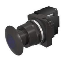
30mm BlackMax, Epoxy Coated Corrosion Resistant Complete Metal Unit Illuminated Push-Pull Operator Transformer type, 600V AC Incandescent Lamp Mushroom Head Cap Small 1 3/4" (44.5 mm) Metal, Black with Blue Lens 2 Position Maintained, Pull-to-Release UL Listed, CSA Certified NEMA 1,3,3R,4,4X,12,13 & Automotive Standards
