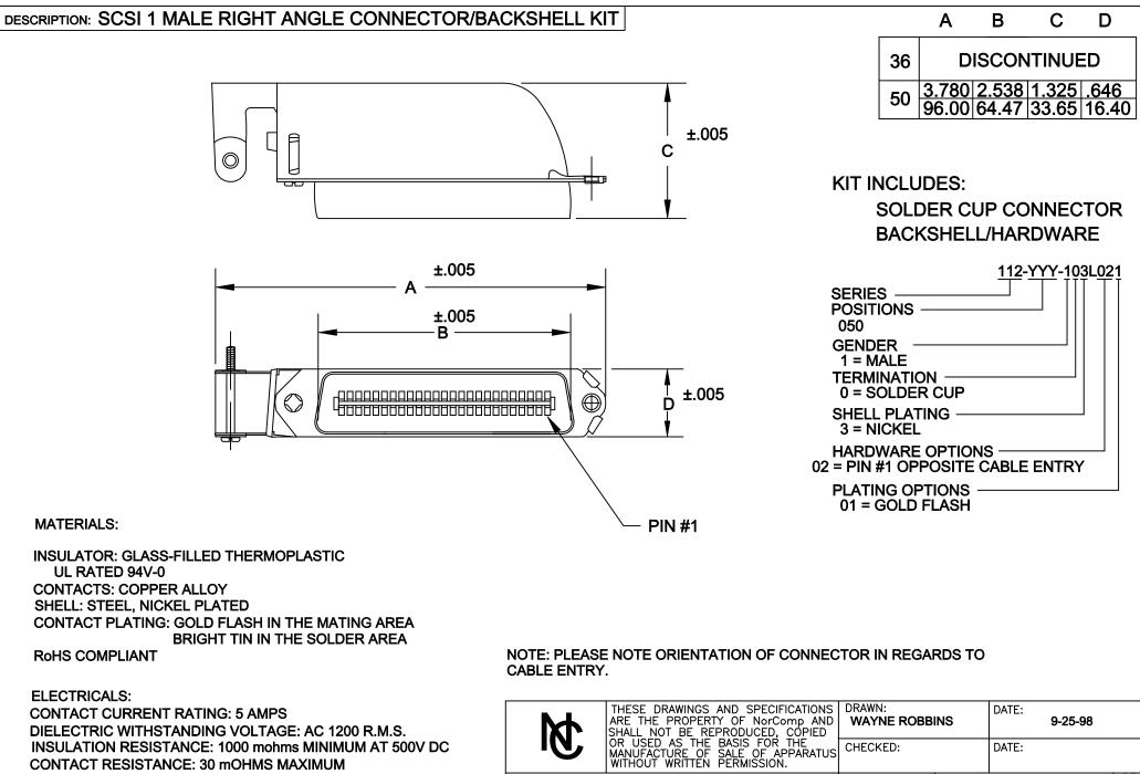
INSULATION RESISTANCE: 1000 mohms MINIMUM AT 500V DC
