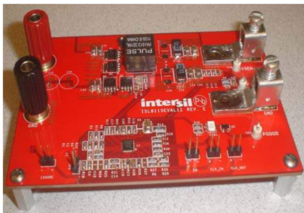
FIGURE 1. ISL8115EVAL1Z EVALUATION BOARD
