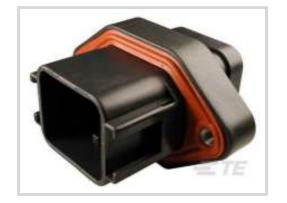
Connector & Housing Type: Housing for Male Terminals Mating Pin Diameter: 1.59 mm [.063 in ] Connector System: Wire-to-Wire Number of Positions: 18 Centerline (Pitch): 4.45 mm [.175 in ]
