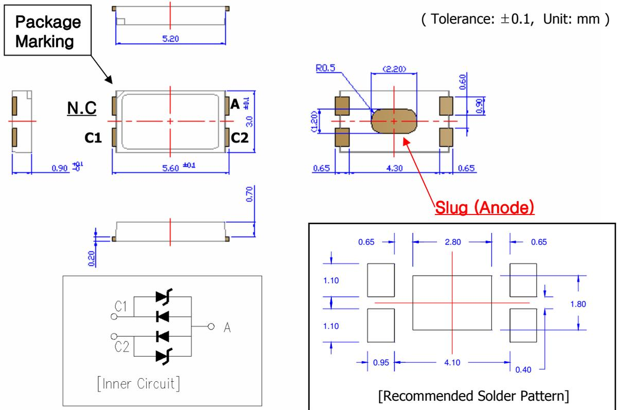
[Note] Forward current is 50mA per die for parallel inner circuit.
