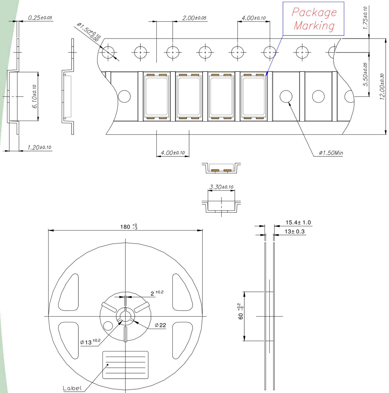
( Tolerance:  $\pm 0.2$ , Unit: mm )
