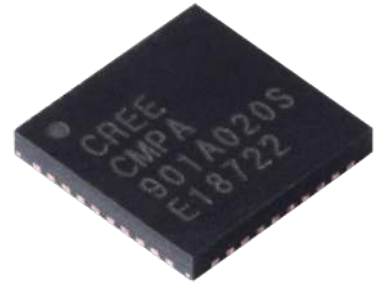
PN: CMPA901A020S Package Type: 6x6 QFN
