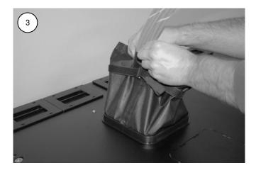
Step 3: Seal the hook and loop strip along the top edge of the fabric sleeve
