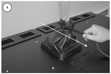
Step 4: Pull the cinch tie tight around the cable bundle as shown. Wrap the cinch tie around the cable bundle and attach it to itself. If applicable, trim off excess cinch tie material.
