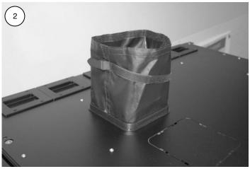
Step 2: With the fabric of the cool boot opened up, route the cable bundle through the opening.
