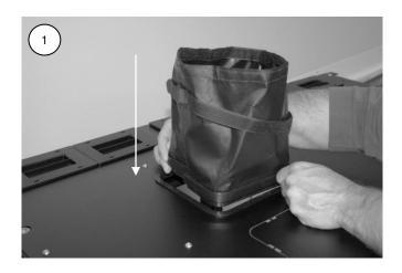
Step 1: Install Cool Boot by pressing down on top of the outer edges of the fitting assembly.
