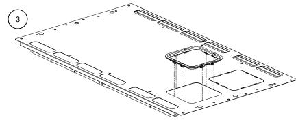
Step 3: Insert bezel into top of cabinet by snapping into place over each latch. Visually inspect to ensure all latch tabs have engaged below the opening.
