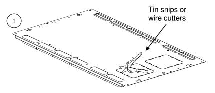
Step 1: Using tin snips or wire cutters, cut the (8) tabs and remove cut-out from top of cabinet.
