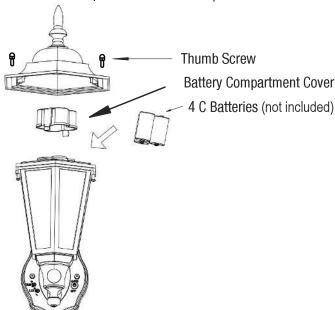
2. Remove the battery compartment cover by squeezing the two tabs on the cover inward and pulling up.
