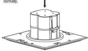
5. Reassemble the LED Outdoor Wall Sconce by replacing the top cover and re-installing the two thumb screws. Tighten the thumb screws by hand as tightly as possible to ensure a waterproof seal.
