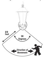
The motion sensor has a detection area of about 23 feet (7 meters) within a 90 degree angle of the sensor. The sensor is more sensitive to movement across the detection area than movement directly towards or away from the sensor.
