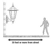
Ideally, the *LED Outdoor Wall Sconce* should be mounted with the detector at the height of or above the objects to be detected.
