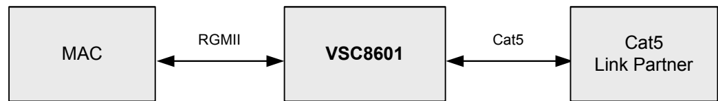
Figure 3. RGMII to Cat5 Block Diagram
