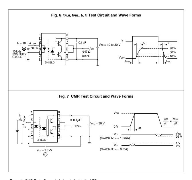
$\textbf{Remark} \quad \text{CMR Test}: \text{Connect pin 1 and pin 4 to the LED common}.$
