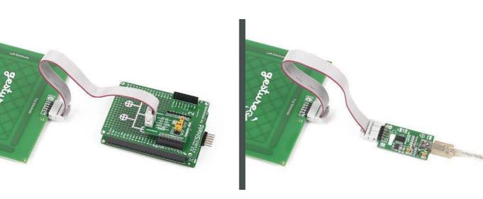
The Gesture board comes with an IDC10 connector cable. If you wish to use it for hardware prototyping, we suggest you pair it with adapter click. The other options is to develop PC applications. For that purpose we developed the Gesture USB adapter.
