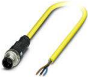
Sensor/Actuator cable, 3-position, TPE, yellow RAL 1021, Plug straight M12 SPEEDCON, A-coded, on free cable end, Cable length: 10 m
