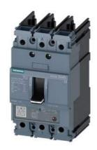
circuit breaker 3VA5 UL frame 125 breaking capacity class M 35kA @ 480V 3-pole, line protection TM230, FTAM, In=110A overload protection Ir=110A fixed short-circuit protection Ii=5...10 x In UL 489 SB (naval), 50° C without connection
