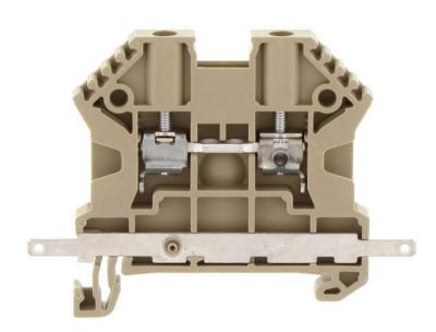
Feed-through terminal, Screw connection, Mounting type: Mounting rail TS 35/7.5, Rated cross-section: 2.5 mm², Width: 5 mm, Colour: Black
