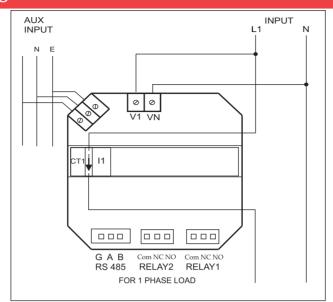
It is recommended that the wires used for connections to the instrument should have lugs soldered at the end. That is, the connections should be made with Lugged wires for secure connections. The Maximum diameter of the lug should be 7.0 mm and maximum thickness 3.5 mm.
