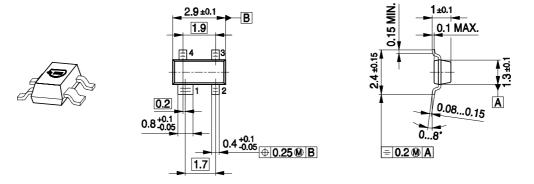
Note: Mold flash, protrusions or gate burrs of 0,2 mm max. per side are not included
