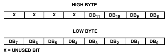
Figure 38. Data Format for AD5341
