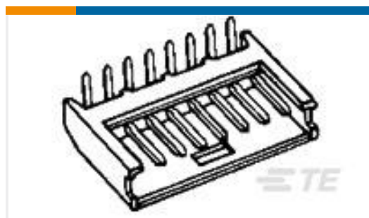
TE Part #280365 AMPMODU, DBL ROW, CONTACT REC
