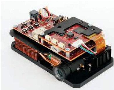
Figure 9. DLP LightCrafter Display Complete EVM
