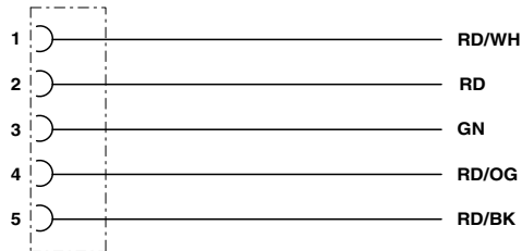
Contact assignment of 7/8" plugs/sockets, cable type 420
