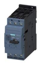
Circuit breaker size S2 for transformer protection A-release 54...65 A N-release 1040 A screw terminal Standard switching capacity
