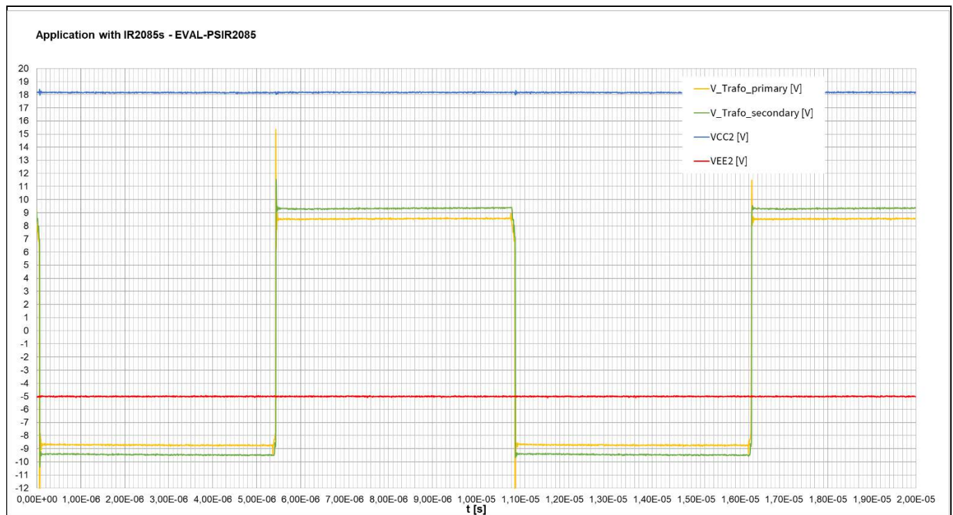
Figure 11 Normal operation of the power supply board
