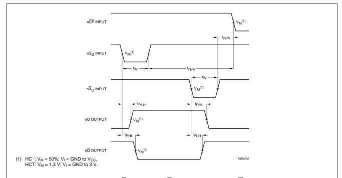
Fig.7 Waveforms showing the set  $(n\overline{S}_{\underline{D}})$  and reset  $(n\overline{R}_{\underline{D}})$  input to output  $(nQ, n\overline{Q})$  propagation delays, the set and reset pulse width and the  $n\overline{R}_{\underline{D}}$  and  $n\overline{S}_{\underline{D}}$  to  $n\overline{CP}$  removal time.
