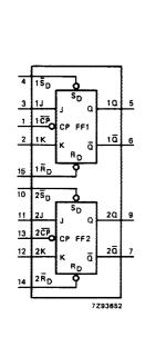
Fig.4 Functional diagram.
