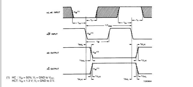
The shaded areas indicate when the input is permitted to change for predictable output performance.
